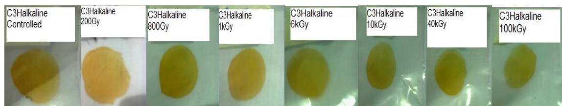
Figure 27. Photographs of Henna C3 alkaline sample films showing decoloration at different doses.
