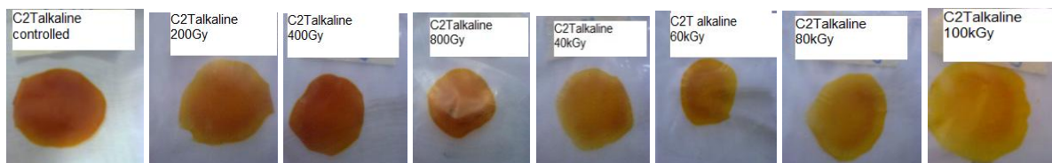
Figure 25. Photographs of Turmeric C2 alkaline sample films showing decoloration at different doses.
