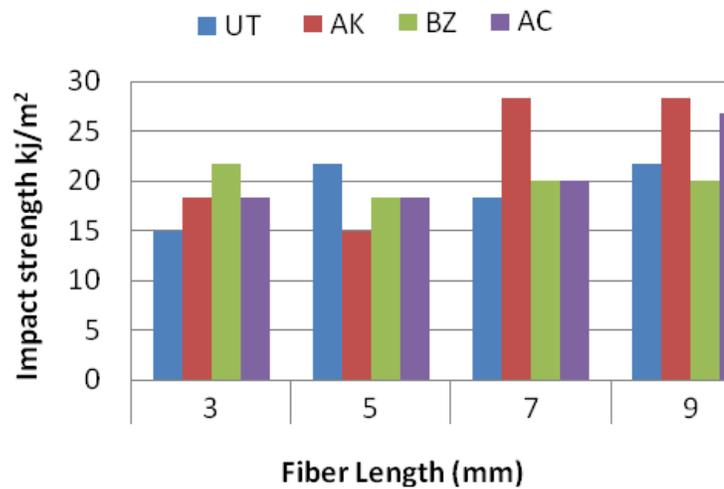
Figure 3. Impact strength versus fiber length.
